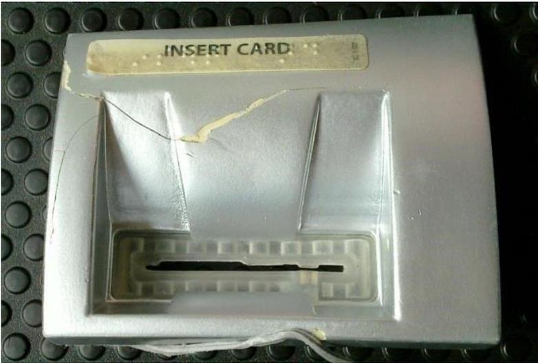
ATM skimmers are becoming more and more sophisticated. Instead of a device fitted over a card slot, a skimmer may be a small, unnoticeable device inserted into the card slot itself.
